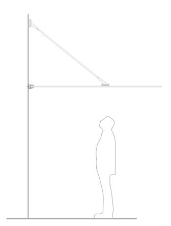
The glassboard is supported by a uniform beam of Salinox's crystal railing bases (depending on the projection distance and glass thickness).
