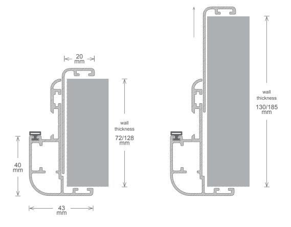
Elegant internal glass doors which consist of a detachable, adaptive oval shaped aluminum profile, serving as the door's frame and capable of embracing walls from 7cm up to 12.5cm in thickness and from 12.5cm up to 18cm in width.
